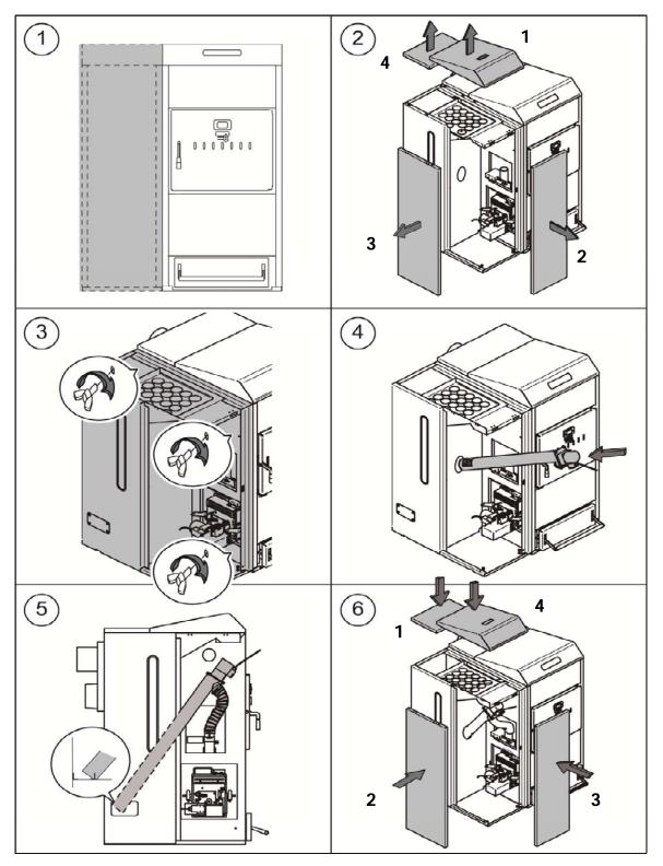
NOTE: The screws to fasten the hopper with the boiler are contained in the documentation bag.
