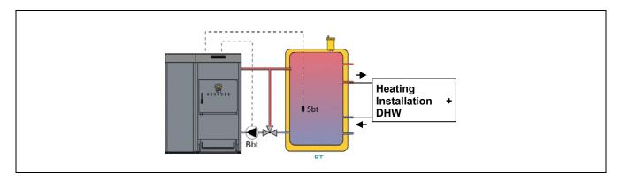
After the hydraulic installation of all the system components, proceed as follows to carry out the correct electrical connection of the BT buffer tank to the **DualTherm** boiler:
