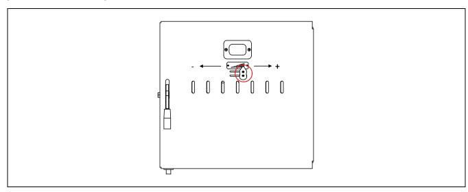
To regulate the air intake, slide the door regulator to the right or to the left depending on the amount of air you wish to supply to the burning furnace.
