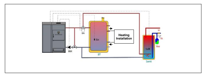
After the hydraulic installation of all the system components, proceed as follows to carry out the correct electrical connection of the BT buffer tank to the **DualTherm** boiler:
