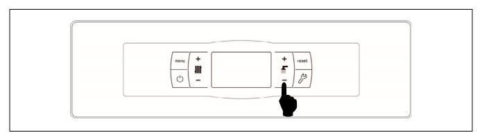
DHW temperature set point selection is made by the tactile selector shown in the picture. Press "+" and "-" buttons to increase or decrease the set point desired. Few seconds after the desired set point temperature is adjusted the display returns to main position. The range of values for DHW temperature set point is OFF, 15 - 65 °C.
