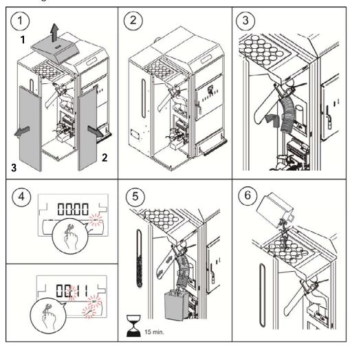
IMPORTANT: It is compulsory to fill the feed auger during the commissioning or when the hopper runs out of fuel.
