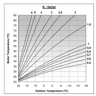
Depending on the type of heating circuit, isolation of the building and position of the outdoor sensor, the optimal K-factor curve could be different. Nevertheless, a general rule could be that for high temperature heating circuits (radiators heating circuit) the K-factor curve should to be 1 or higher and for low temperature heating circuits (under floor heating circuit) it should be 0.8 or less.
