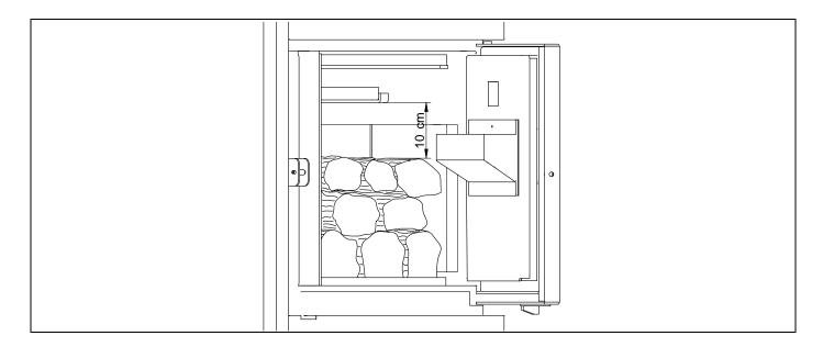
Always put at least four logs at a time. It is advisable to add small wooden slats when using large firewood logs and/or with more moisture. Put at least one of those logs over the burner.
