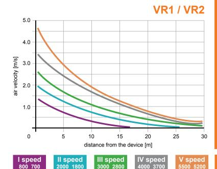
The chart presents the ranges of airflows to the point where the speed in the airflow axis is 0.5 m/s (recommended speed in the occupied zones for the industrial sites) in relation to the place of installing the unit horizontally on the wall and to the position of the direction louvers.
