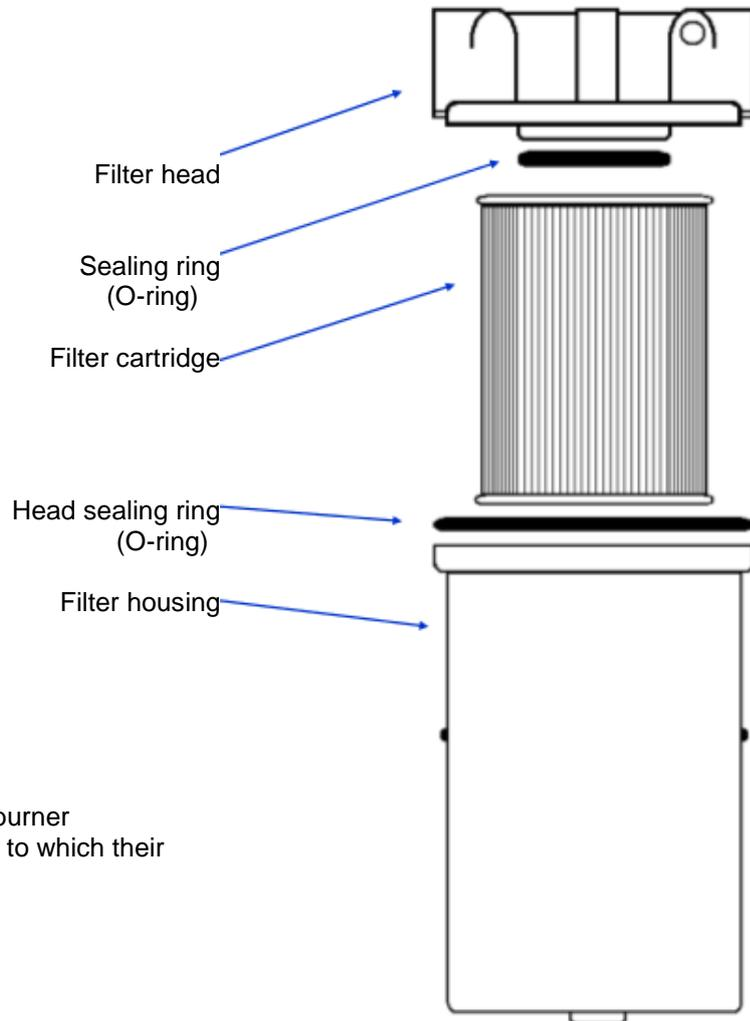
**Warning!** Oil filters recommended by the burner manufacturer, MTM, are washable, thanks to which their cartridges may be reused.
