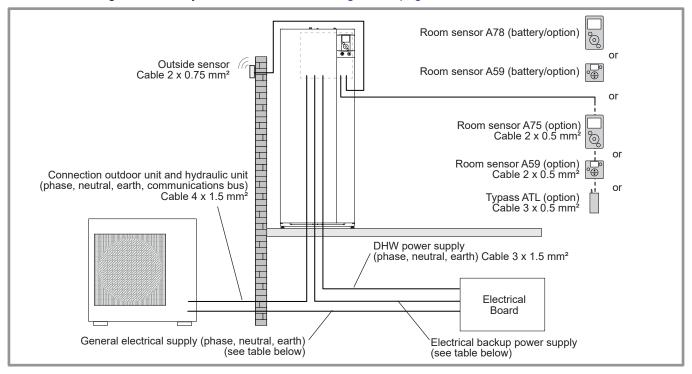
figure 33 - Overall layout of electrical connections for a simple installation (1 heating circuit)
