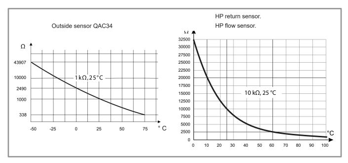
figure 6 - Ohmic sensor values (Hydraulic unit)
