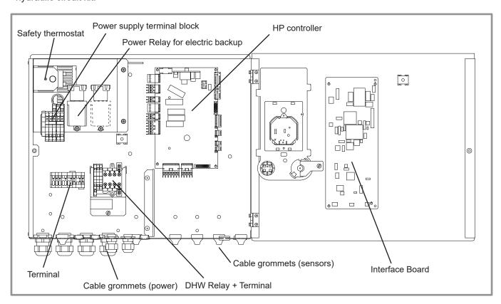
figure 36 - Description of the hydraulic module's electrical control box
