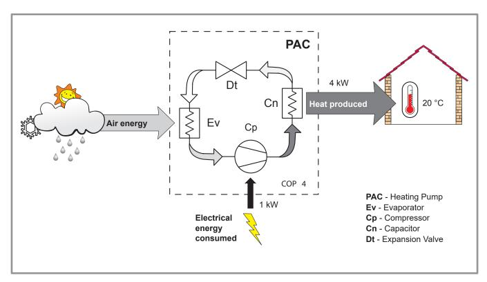
figure 11 - Heat pump operating principle
