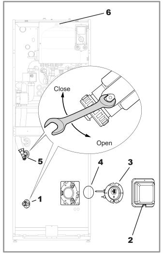
figure 49 - Draining the hydraulic unit
