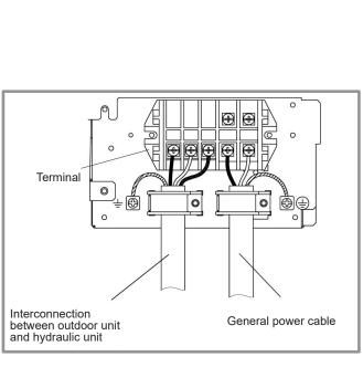
figure 34 - Connections to outdoor unit's terminal block
