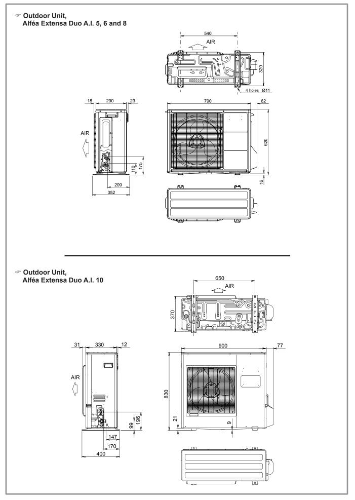
figure 1 - Dimensions in mm
