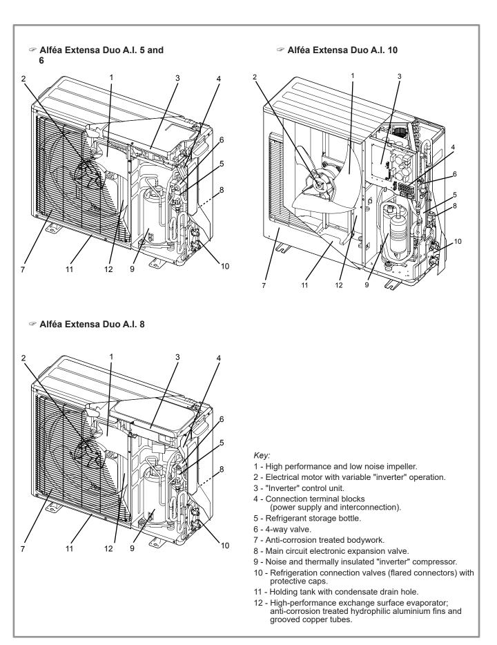
figure 8 - Outdoor unit components
