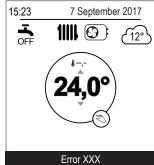
☐ In the event of an error originating in the outdoor unit, the user interface displays error code "370: Thermodynamic Generator" followed by the outdoor unit error.
