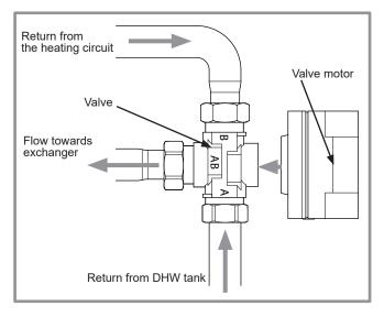
figure 50 - Mounting the distribution valve
