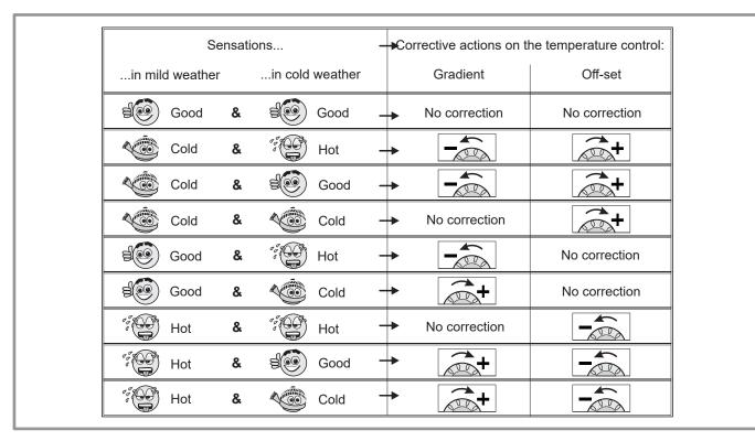
figure 44 - Corrective actions in case of discomfort
