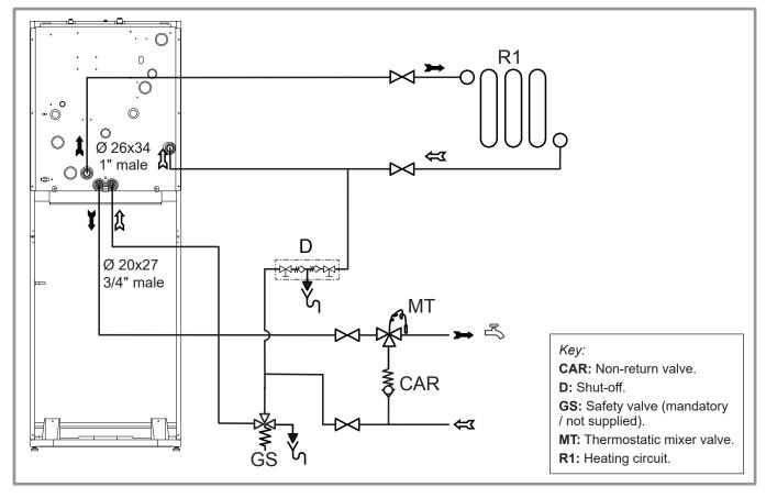
figure 25 - Basic Hydraulic Layout
