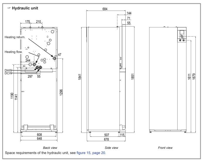
figure 2 - Dimensions in mm
