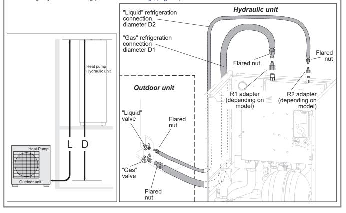
figure 19 - Refrigeration connections (authorised diameters and lengths)
