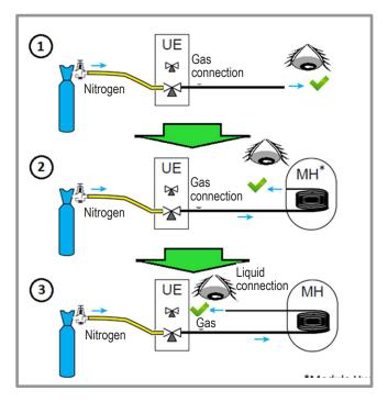
figure 21 - Checking refrigeration connections
