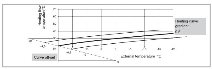
figure 43 - Transferral of the heating curve
