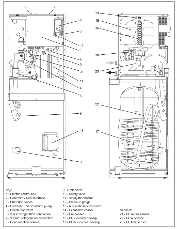
figure 9 - Hydraulic unit components
