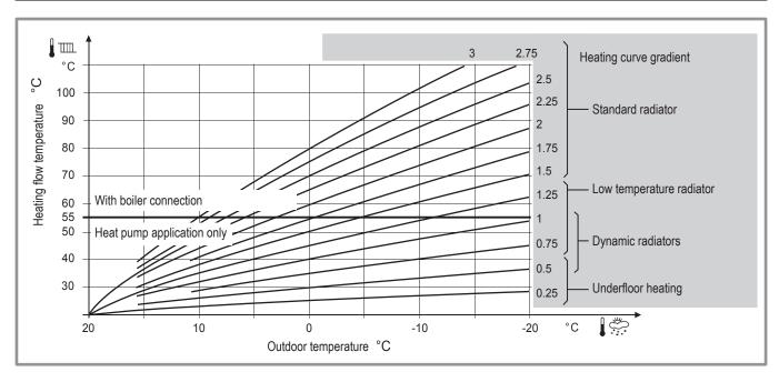
figure 42 - Heating curve gradient
