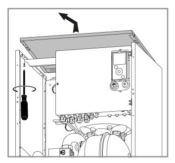
figure 17 - Removing the cover
