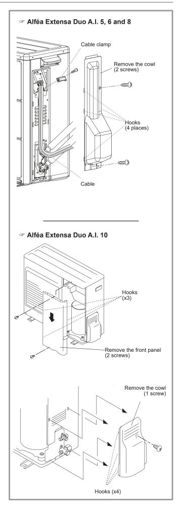
figure 35 - Access to outdoor unit's terminal block
