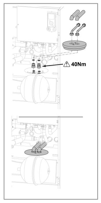
figure 26 - Attaching DHW pipe connections
