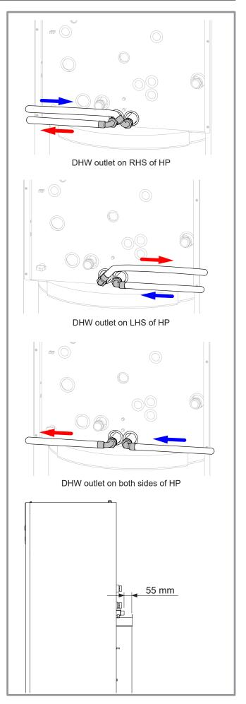
figure 27 - DHW circuit outlets
