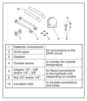
figure 4 - Accessories provided with the hydraulic unit
