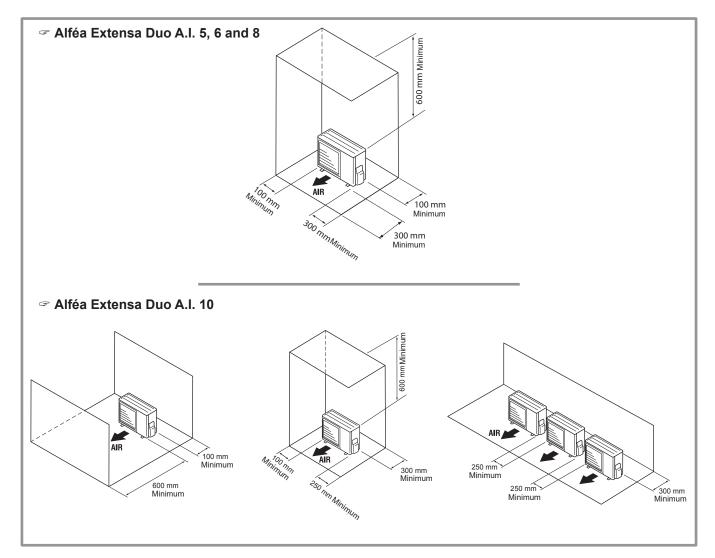
figure 13 - Minimum installation clearances around the outdoor unit
