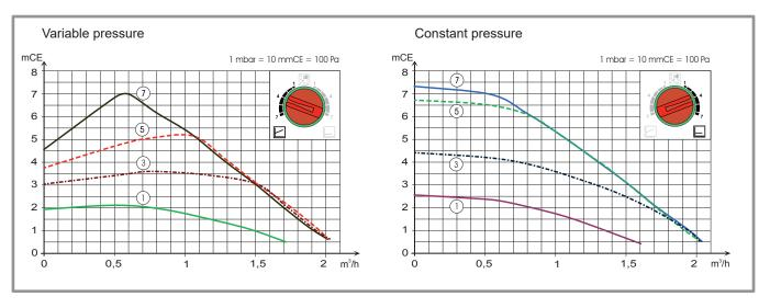
figure 5 - Available hydraulic pressures and flow rates
