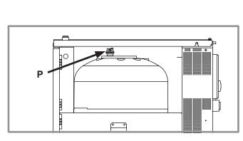
figure 29 - Hydraulic unit automatic bleeder valve
