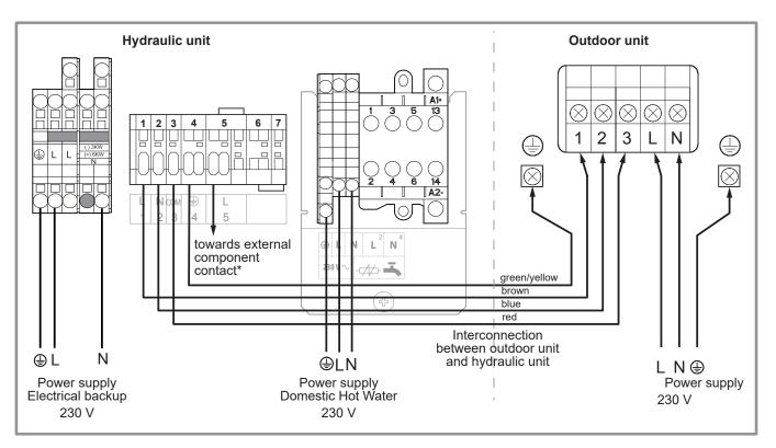
figure 37 - Connection to terminal blocks and power relay
