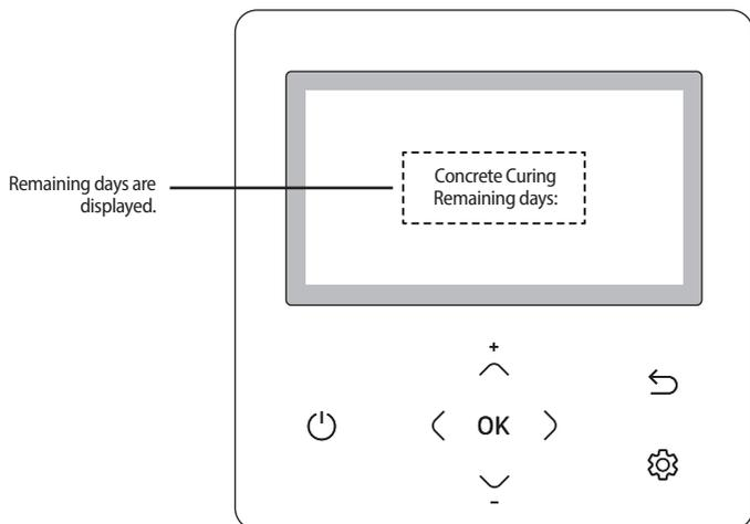
\* If an error is displayed, concrete curing function does not work.
