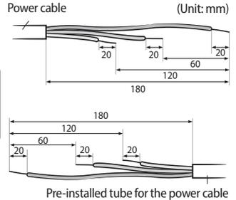
3. Insert both sides of core wire of the power cable into the connection sleeve.
