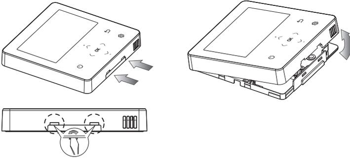
2. Arrange the power cable and the communication cable so that they fit in the housing along the edges of the rear cover.
