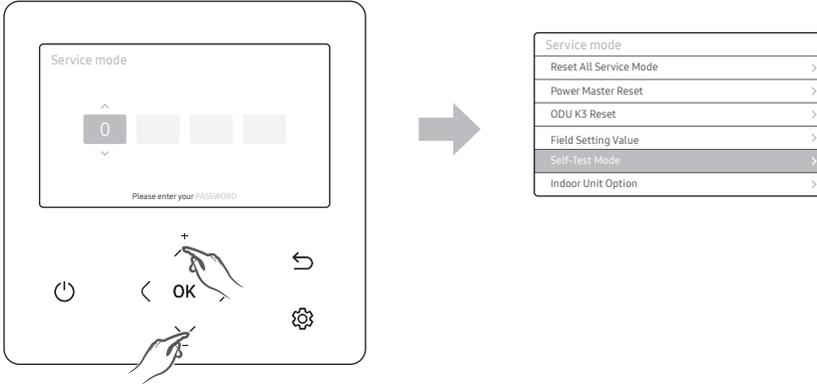
1. If you want to use the various additional functions for your Wired Remote Controller, press the  $\wedge$  and  $\vee$  buttons at the same time for more than 3 seconds.
