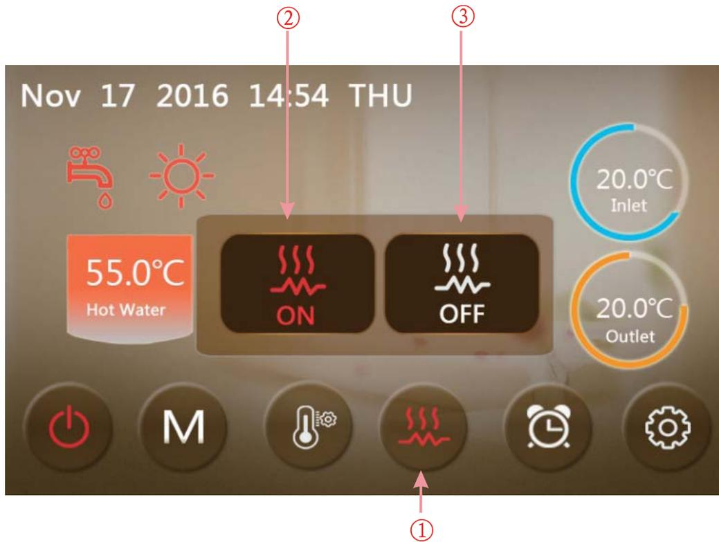
Under the heating mode, click the fast heating key ① the above interface will appear. Click ② to start the fast heating and click ③ to close it.
